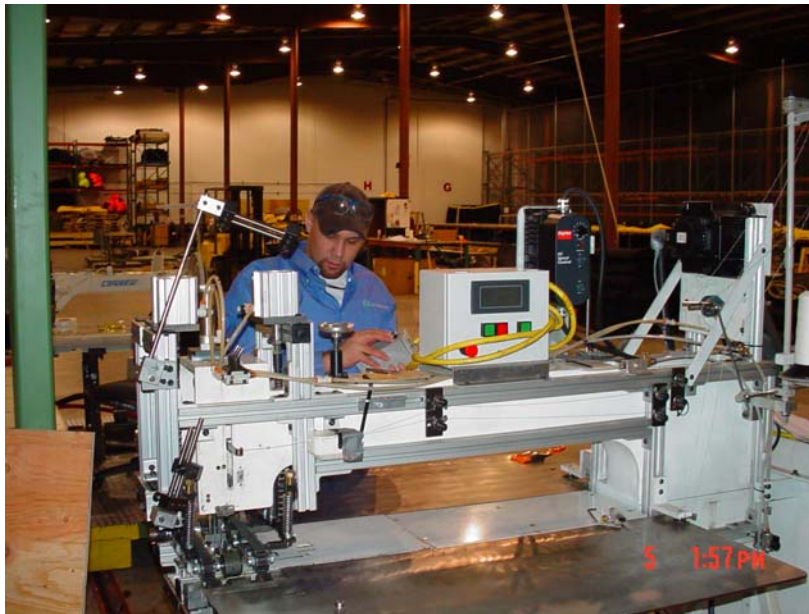
Figure 7. Gunderboom's custom-manufactured sewing machines are capable of sewing through thick layers of filter fabric, reinforced skirt fabric and 10,000-pound nylon support strapping.
