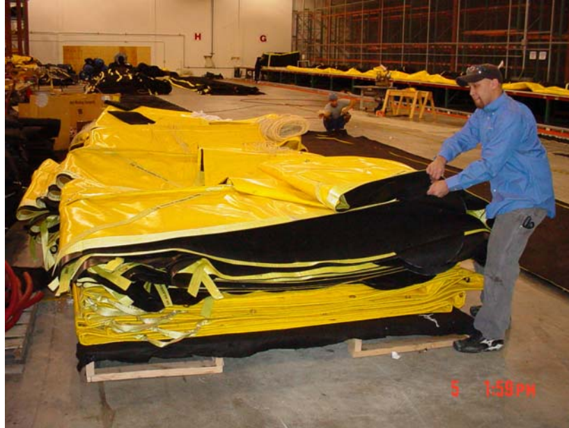
Figure 8. After the manufacturing process is complete, sections, many on the order of 140-feet long and complete with hood, fabric, impermeable skirt, nylon webbing, structural netting, anchor attachment points, air hoses, bottom chain and more, are loaded onto pallets for shipping to the site.
