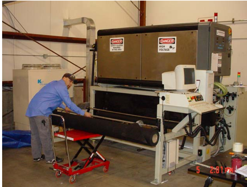
Figure 7. Gunderboom's custom-manufactured sewing machines are capable of sewing through thick layers of filter fabric, reinforced skirt fabric and 10,000-pound nylon support strapping.
